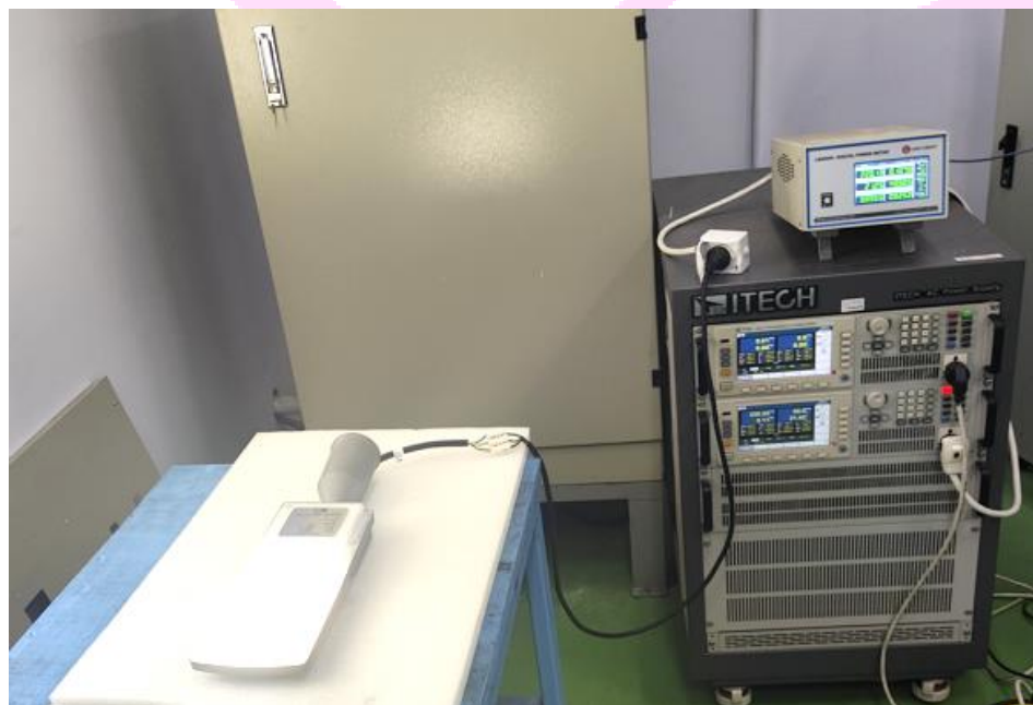
Figure 1 - Test Setup of Harmonic Current Emissions
