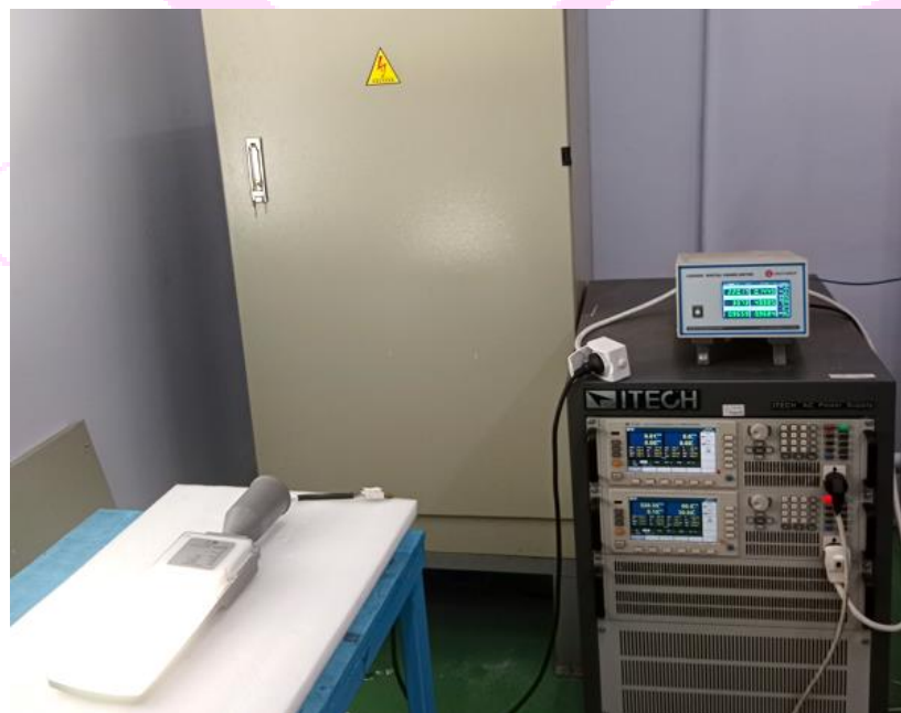
Figure 1 - Test Setup of Harmonic Current Emissions
